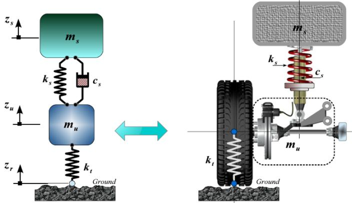
Figure 3.1: A quarter car passive suspension.
