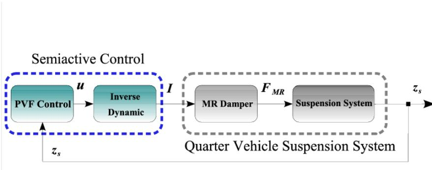
Figure 3.2: Schematic diagram of the semiactive control scheme.
