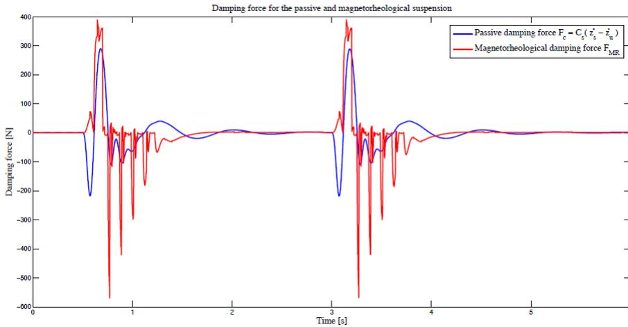
**Figure 3.5:** Damping force for passive suspension ( $F_c = c_s(\dot{z}_s - \dot{z}_u)$ ), and the suspension with MR damper ( $F_{MR}(\dot{v}, I)$ ).
