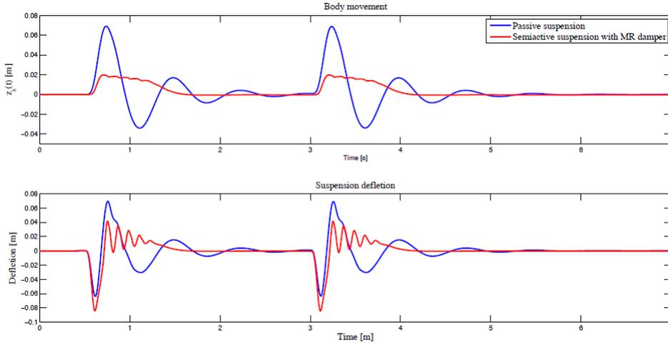
**Figure 3.4:** Simulation results of the passive suspension ( $F_c = c_s(\dot{z}_s - \dot{z}_u)$ ), and using a MR damper ( $F_{MR}(\dot{v}, I)$ ).
