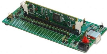
Figura 4.3: TMS320F28069 Experimenter C2000, Piccolo C28x MCU 32 bits.
