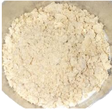
Figure 18. Powder rich in phenolic compounds obtained from the freeze drying of the nanofiltration retentate.
