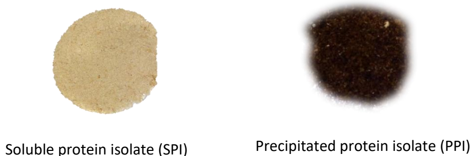
Figure 16. Powders of soluble protein isolate (SPI) and precipitated protein isolate (PPI) obtained in black quinoa by ultrafiltration.
