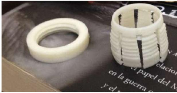
Figura 3.33: Prototipo de ABS Rapid prototyping.
